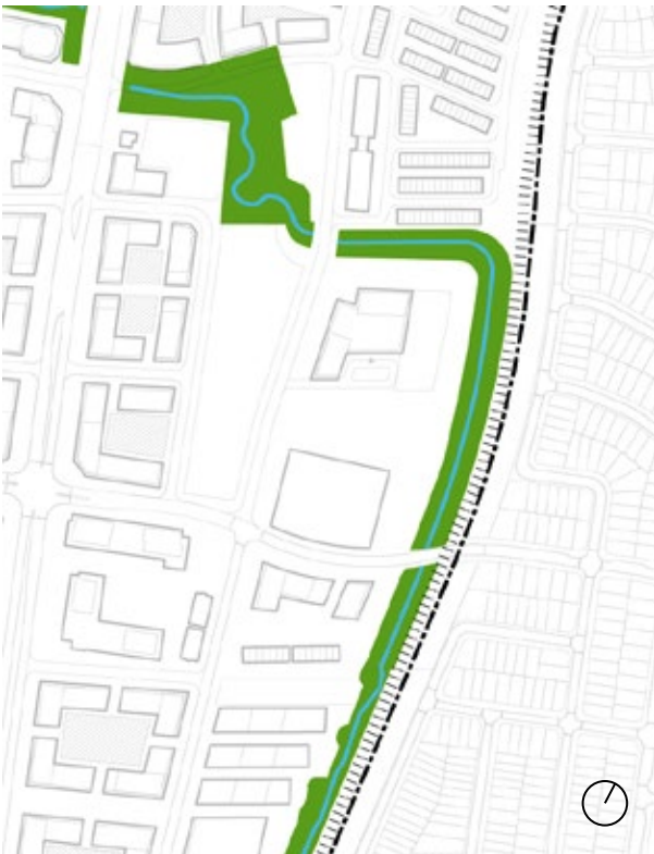
Figure 52: Option 3: Open Channel Along the Proposed and Existing Anderson Avenue Alignment
