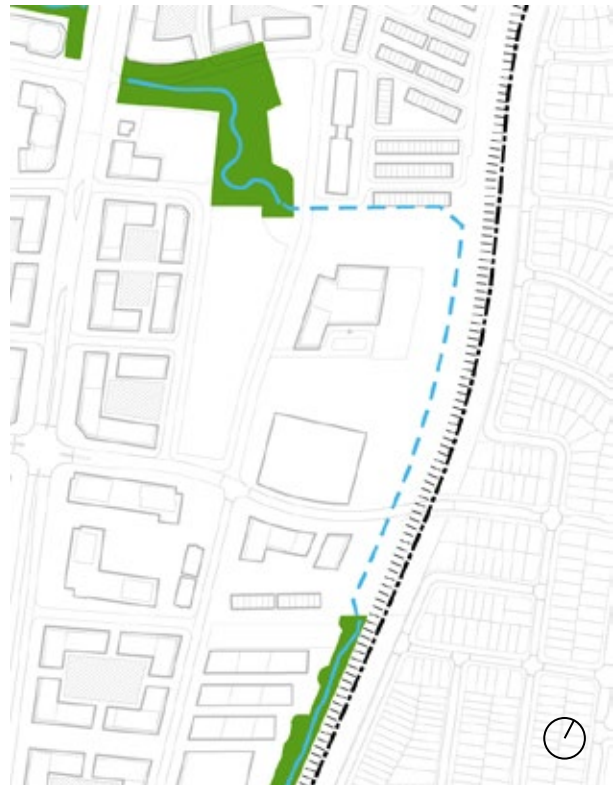
Figure 53: Option 4: Piped System Adjacent the Proposed and Existing Anderson Avenue Alignment
