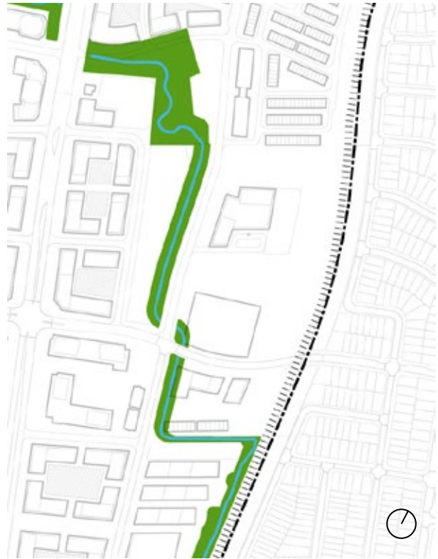
Figure 51: Option 2: Open Channel Adjacent the Proposed and Existing Anderson Avenue Alignment
